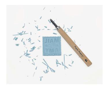
4. Now use the **carving tools** to carefully expose the **motif** bit by bit. First of all circumvent the motif with a **gouge**. Use the **small gouges** to work out fine lines and details. Then use the **flat irons** to cut clear edges and borders. The carving depth should be about **2 - 3 mm**
