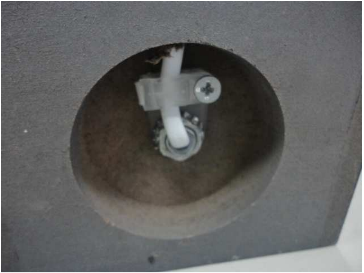
Cord anchorage inside lampholder
