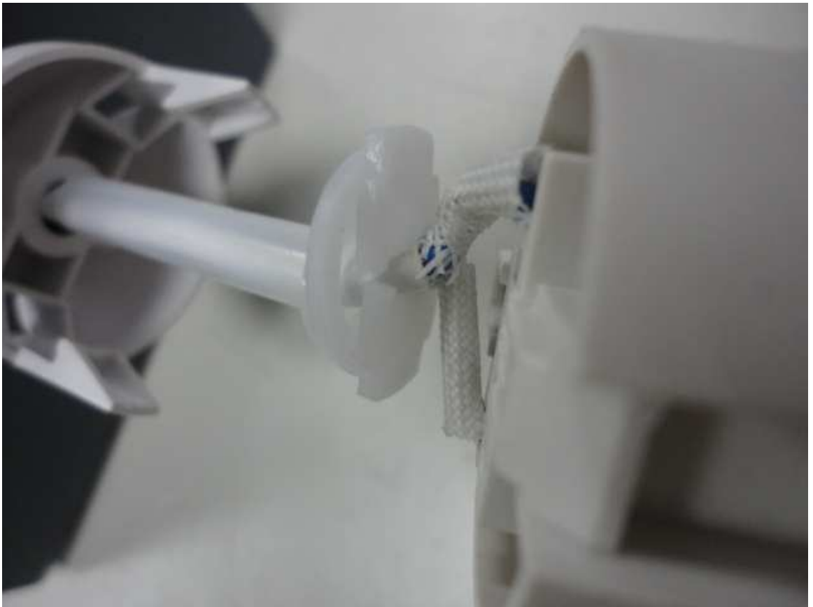
Cord anchorage inside lampholder
